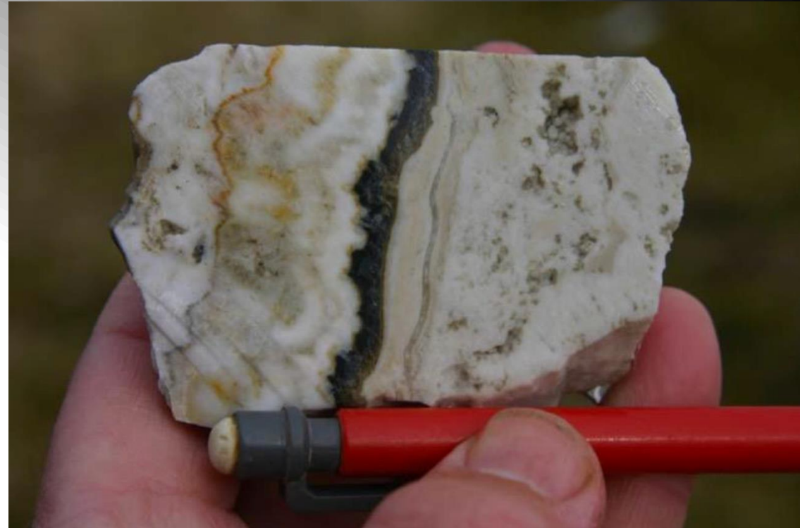
Finely banded chalcedony vein with black sulphide bands (host to gold mineralisation) @ Þormóðsdalur
